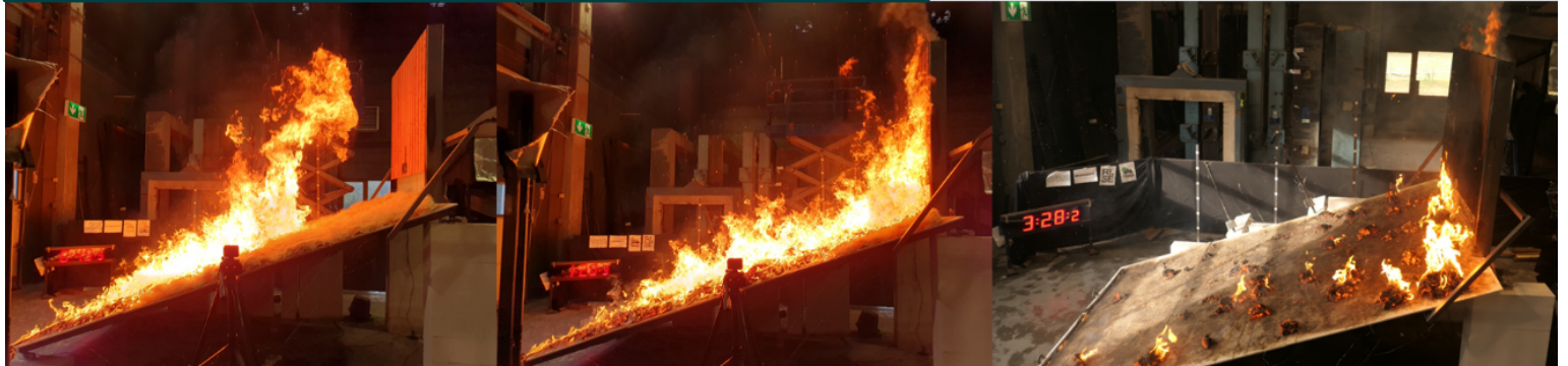
Fire treated wood: No sustained flaming
